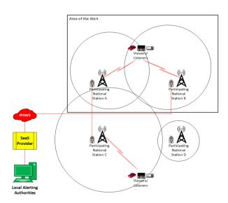
Stations A, B and C receive the alert because they broadcast into the affected county, station D does not.
