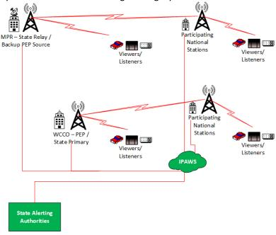
The secondary "legacy" method uses leased lines to send an audio message to the State Primary (SP) WCCO-AM and State Relay (SR) Minnesota Public Radio (MPR) as shown in the diagram below.
